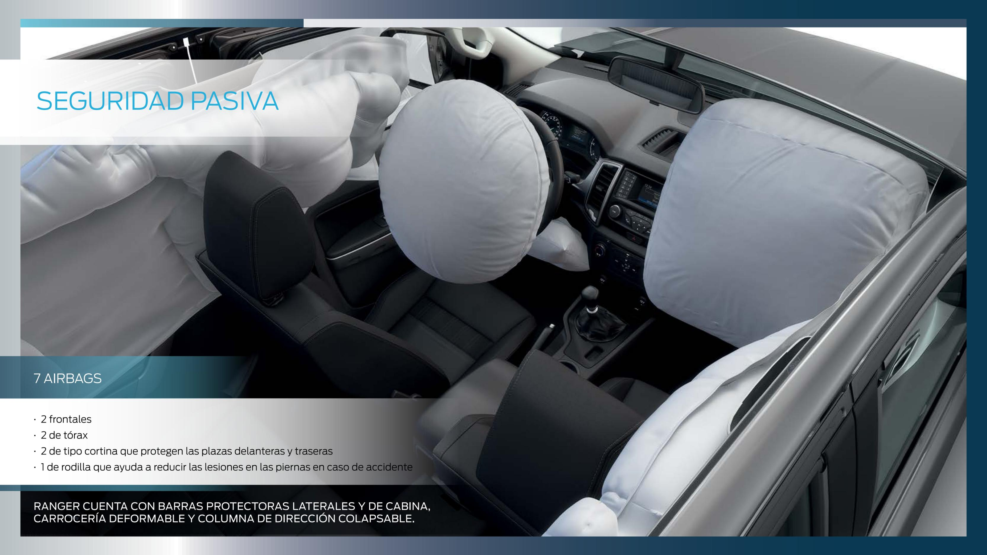
A high-angle photograph of a car's interior with all seven airbags deployed. The driver's side airbag is fully inflated, as is the passenger's. Side-curtain airbags are visible along the outer edges of the front and rear seats. A knee airbag is deployed from the driver's seat. The dashboard, steering wheel, and center console are visible in the background.
